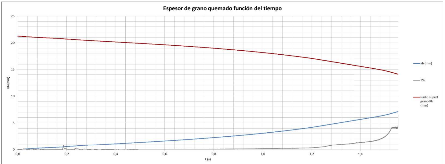
Figure 9: Grain thickness (mm) burnt function of time (s)
