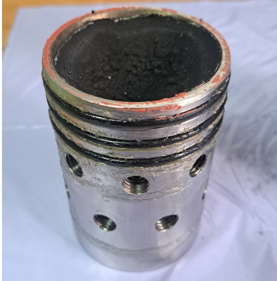
(a) Nozzle with the aluminum layer in the convergent section
