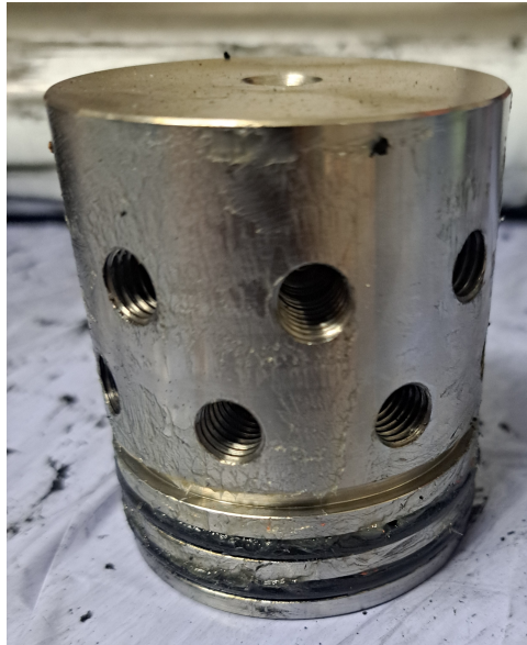
Figure 13: Aft closure of the motor after the test.
