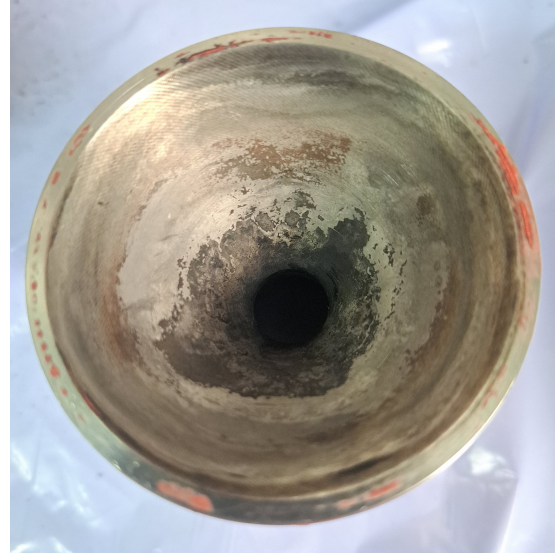
(b) Clean nozzle where the aluminum layer has been removed
