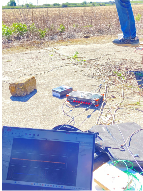
Figure 7: Remote monitoring station located outside the hazard zone. The decentralized architecture ensures human control and real-time parametric visualization without compromising safety.
