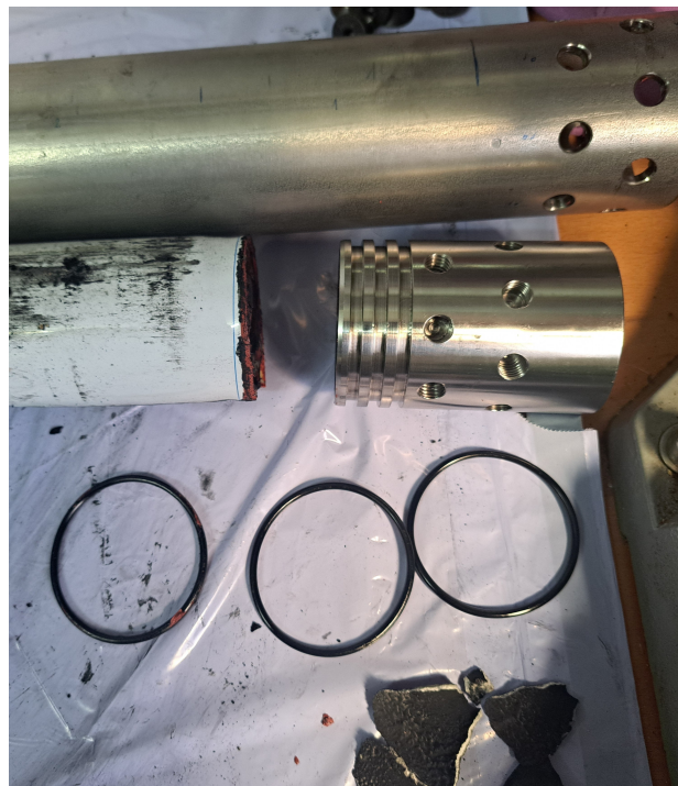
Figure 15: Liner, nozzle, nozzle's O-rings, combustion chamber and removed aluminum crust
