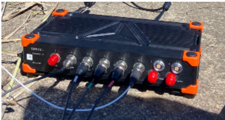
Figure 6: Dewesoft SIRIUS i-CHG deployed in the field. Note the coaxial connections and BNC connectors, which are critical for rejecting electromagnetic interference (EMI) in the test environment.
